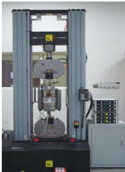
Z150电子式高温拉伸试验机 Z150 electronic elevated temperature tensile tester
